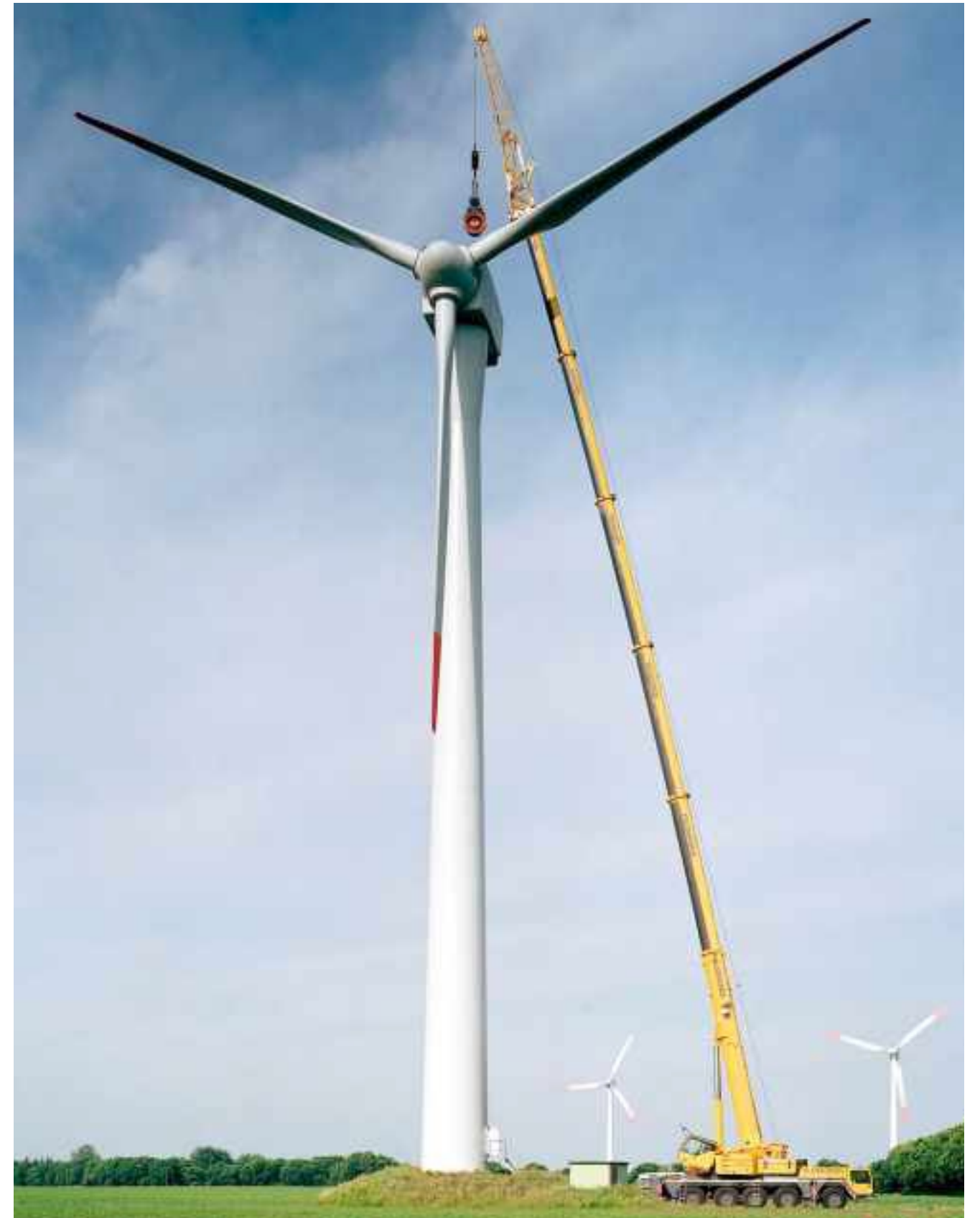
Company: Liebherr – Werk Ehingen GmbH Contact person: Josef Hauser Location: Ehingen, Germany Product: Mobile cranes Material replacement: From WELDOX 960 to WELDOX 1100 Period: 2001 Results: Increased lifting capacity and unchanged crane weight
