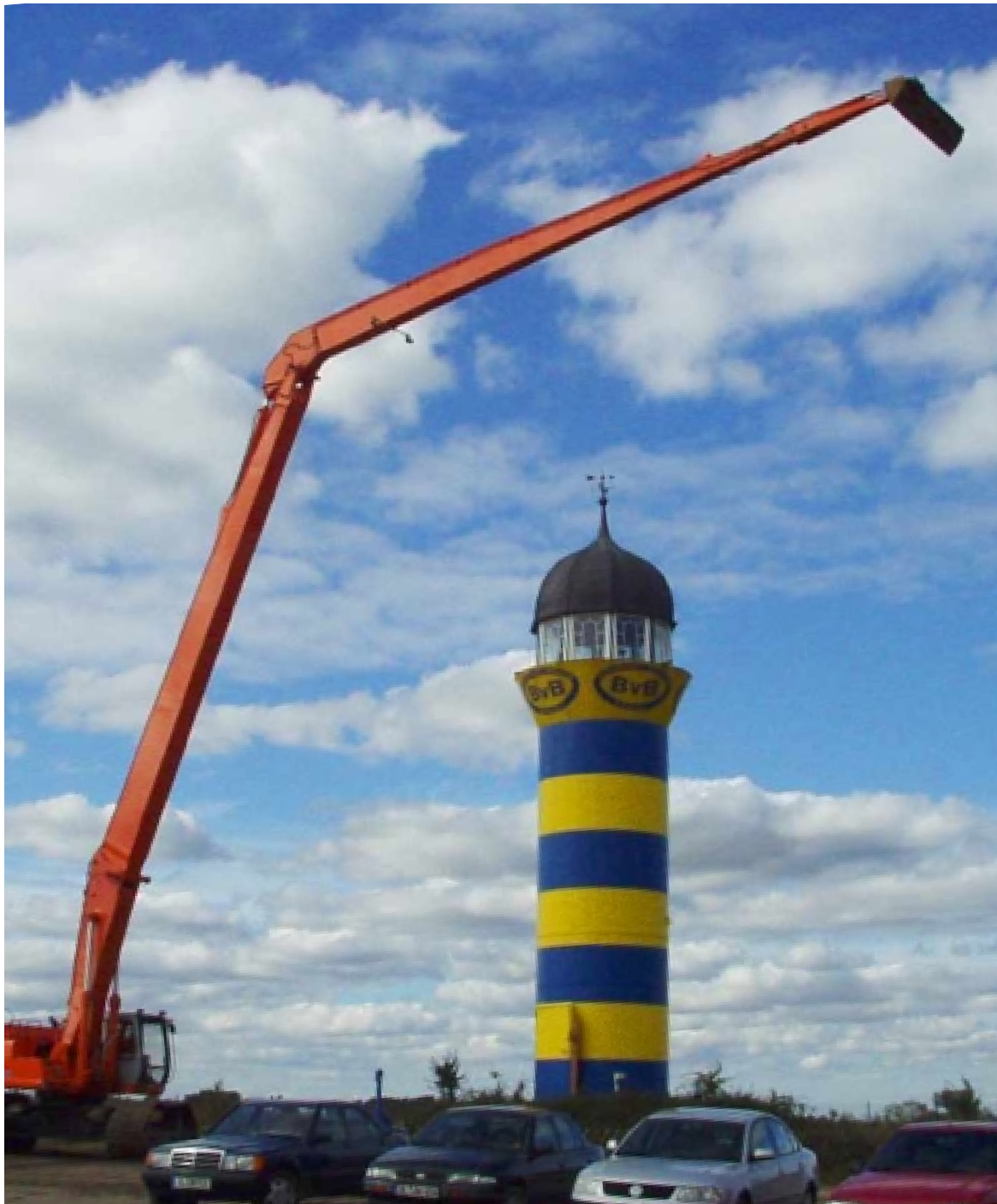
Company: Kocurek Excavators Contact person: David Kocurek Location: Ipswich, England Product: Extra long booms for excavators Material replacement: From S355 to WELDOX 700 and WELDOX 900 Period: Continual upgrading for 10 years Results: Longer booms as the company changes to stronger steel
