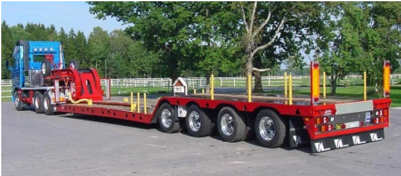
Company: VM Trailer AB Contact person: Peter Lindström Location: Härryda, Sweden Product: Trailers Material replacement: From WELDOX 500 to WELDOX 700 Results: About 10 per cent lower weight
