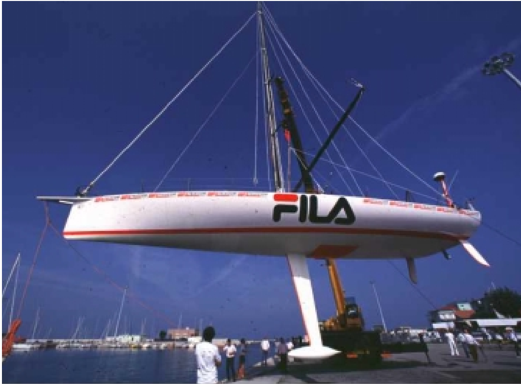
Company: AMPM Contact person: Fabien Dillet Location: La Motte Achard, France Product: Sailboat keels Material replacement: From S355 to WELDOX 1100 Period: 1998-99 Results: Improved weight distribution, static strength and fatigue properties
