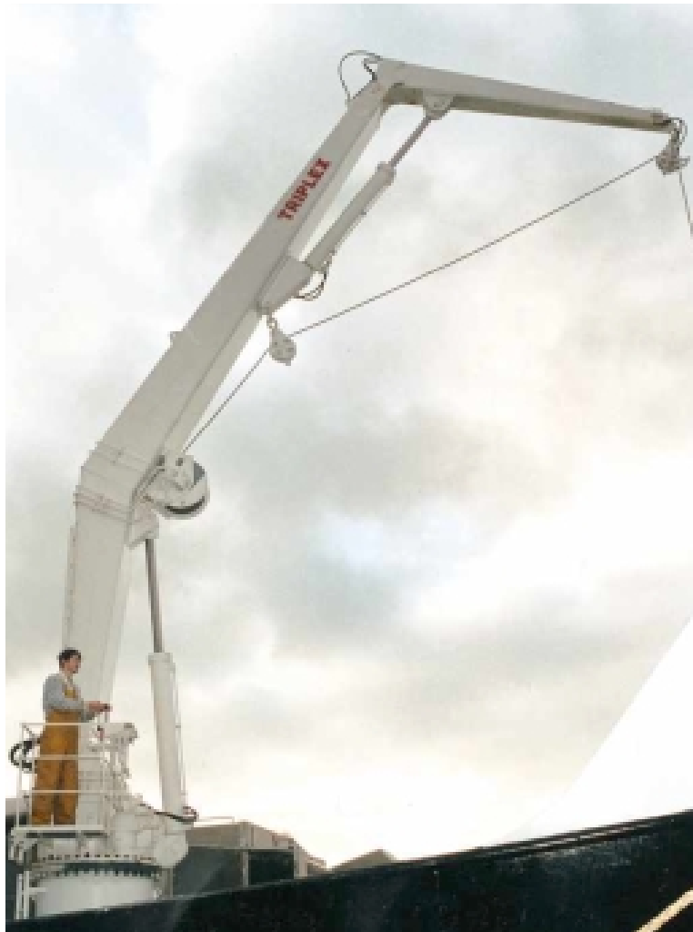
Company: SM TRIPLEX AS Contact person: Jan Geir Kristiansen Location: Averøy, Norway Product: Deck cranes Material replacement: From S355 to WELDOX 700 Period: 2001 Results: 30 per cent lighter crane and base weights enable less ballast to be used, which reduces the vessel draught and fuel consumption
